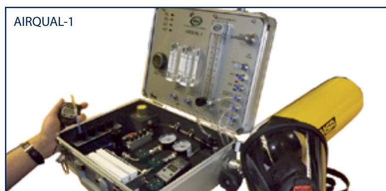
To help you carry out the regular tests, as required by the BS EN12021, a1-cbiss have designed a conveniently packaged breathing air quality test kit that comes with everything required for an ‘on the spot’ test. At 4kg and packaged in an aluminium casing, the **AIRQUAL-1** is rugged, lightweight and does not require charging, meaning that it can even be used in situations where power isn't accessible.
