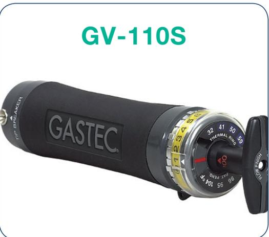
The Gastec Sampling Pump is used in conjunction with Gastec Detector Tubes to draw a sample of hazardous gas across the chemical reagent within the tube such that a change produced is proportional in length to the concentration.
